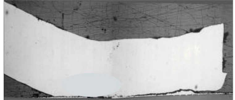
Cross section through Al wire bond failed after power cycling Siepe et al., The Future of Wire Bonding is? Wire Bonding I, CIPS 2010
